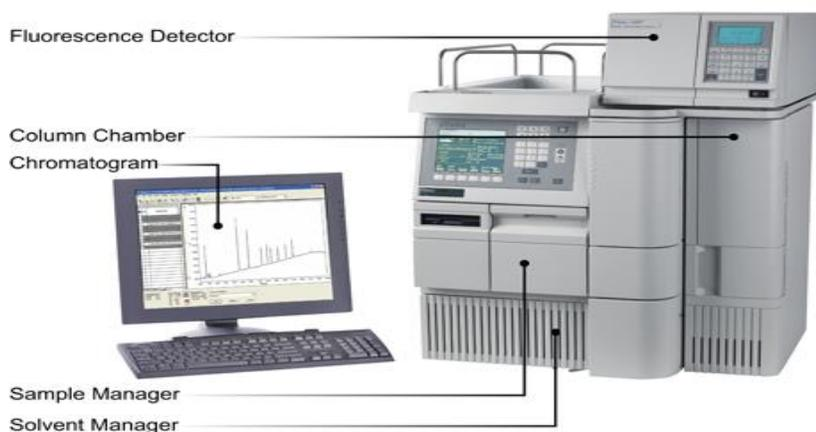
A reservoir holds the solvent [called the mobile phase, because it moves]. A high-pressure pump [solvent delivery system or solvent manager] is used to generate and meter a specified flow rate
