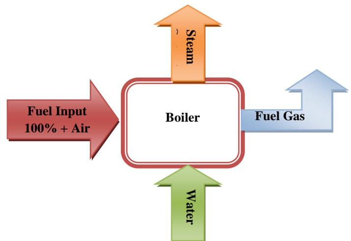
Fig 1: Direct Method for Boiler Efficiency
