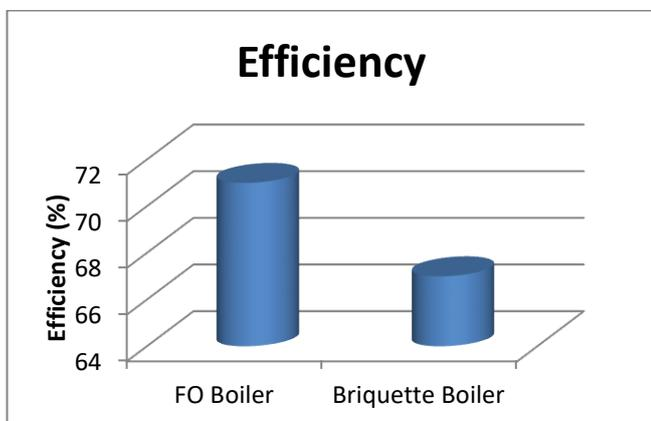
Figure 4: Efficiency Comparison of FO & Briquette Boiler
